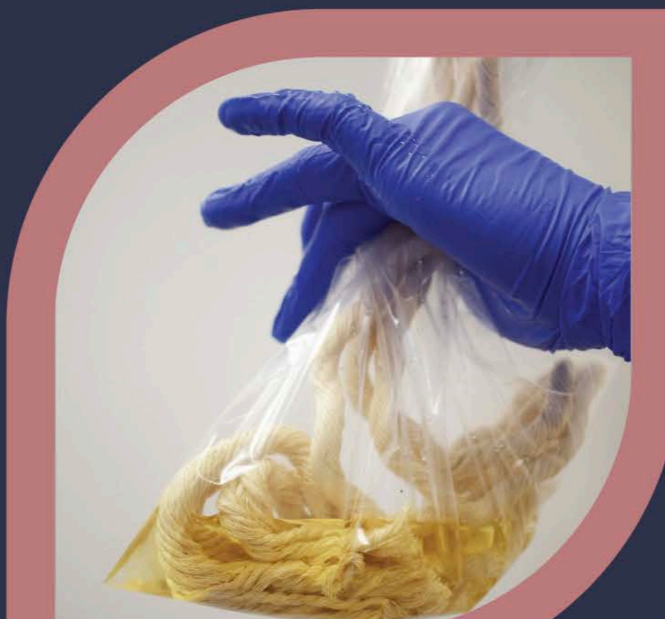
Image 2) Strip the rope so the fluid accumulates in the corner of the bag
